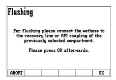
In case the manifold is not empty, it will be drained automatically by the system before the flushing starts. In this mode the pumped volume in liters is shown. The process stops as soon as the manifold becomes empty.
