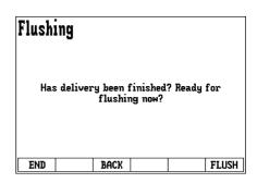
The flushing itself shows a screen, which is very similar to the delivery screen. Only the key page differs, and the flushing progress indicator in the right bottom corner is new ("F=0%").
